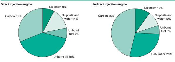
Figure 4.1 Typical Composition of Diesel Exhaust Particulate Matter.
