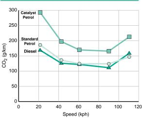
Figure 2.5 Carbon Dioxide Emissions from Different Types of Cars.
