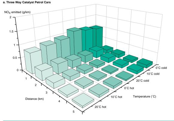
Figure 2.4 Emissions of Nitrogen Oxides with Distance for Hot and Cold Starts in Ambient Temperatures of 0°C, 10°C and 20°C.
