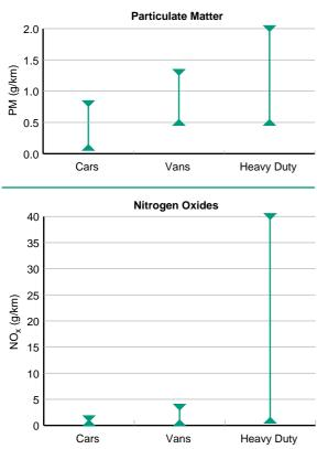
Note: The large range of emissions for heavy duty vehicles reflects the wide range of vehicle types, sizes and technology in this category and the effect of laden weight on emissions, particularly of  $NO_X$ .
