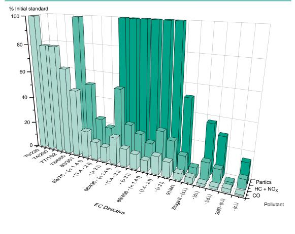
Figure A.1 EC Passenger Car Exhaust Emission Standards 1970-.
