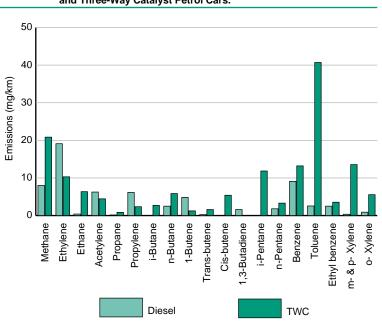
Figure 2.2 Urban Emissions of Individual C1 to C6 Hydrocarbons from Diesel and Three-Way Catalyst Petrol Cars.
