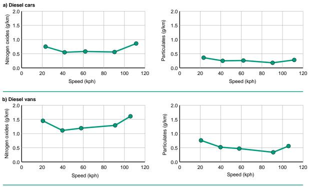
Figure 3.4 Speed Emissions Curves for Diesel Cars and Vans.
