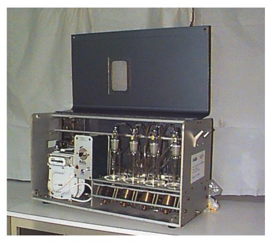
Figure 5.3 8-port Sampler for Smoke and SO<sub>2</sub>
