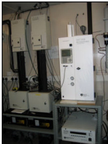
Figure 6: R&P Nitrate 8400N alongside co-located FDMS instruments at Marylebone Road
