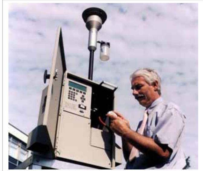
Figure 6. The TEOM instrument for PM 10 , is widely used in the AURN
