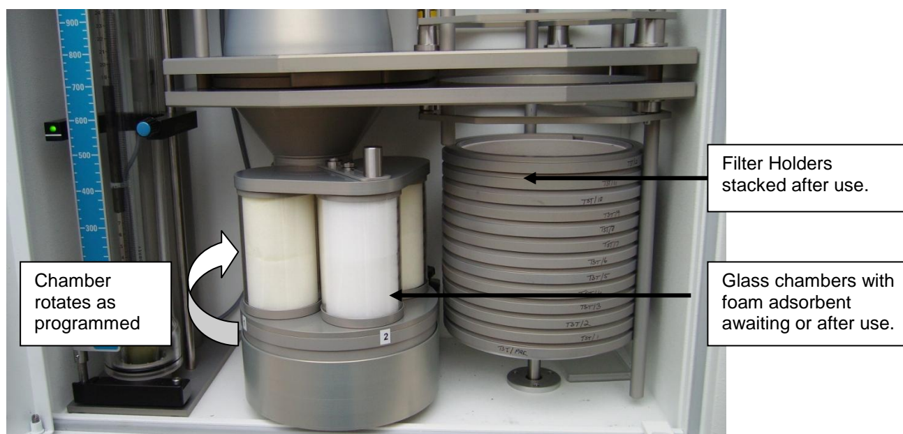
Figure 3: Picture of a Foam Adsorbent Auto Changer for the Digital DHA-80 Sampler
