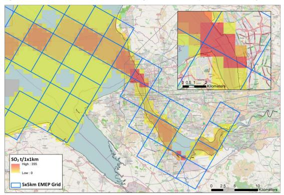
Figure 3.7: SO2 emissions at 1x1km UK grids, overlaid by 5x5 km EMEP grids
