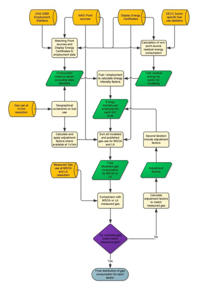
Figure 3.2: Gas consumption modelling data and process flow
