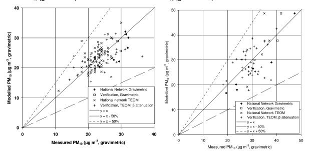
Figure 4.6. Verification of background annual mean PM<sub>10</sub> (gravimetric) model 2006
