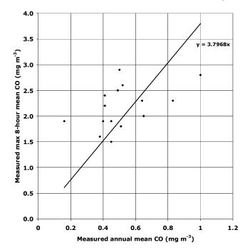
Figure 6.6. Calibration of 2006 roadside maximum 8-hour CO model (mg m<sup>-3</sup>)
