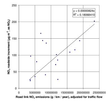
Figure 3.7. Calibration of NO<sub>X</sub> roadside increment model, 2006 (µg m<sup>-3</sup>, as NO<sub>2</sub>)
