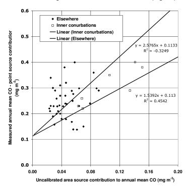
Figure 6.3. Calibration of 2006 background annual mean CO model (mg m<sup>-3</sup>)
