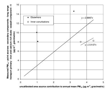
Figure 4.5. Calibration of PM<sub>10</sub> area source model 2006 (µg m<sup>-3</sup>, gravimetric)
