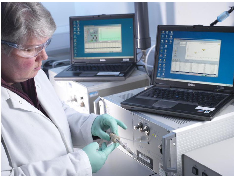
Image 4: Thermal desorption-atomic fluorescence analysers comprising the UK total gaseous mercury analysis facility at NPL.
