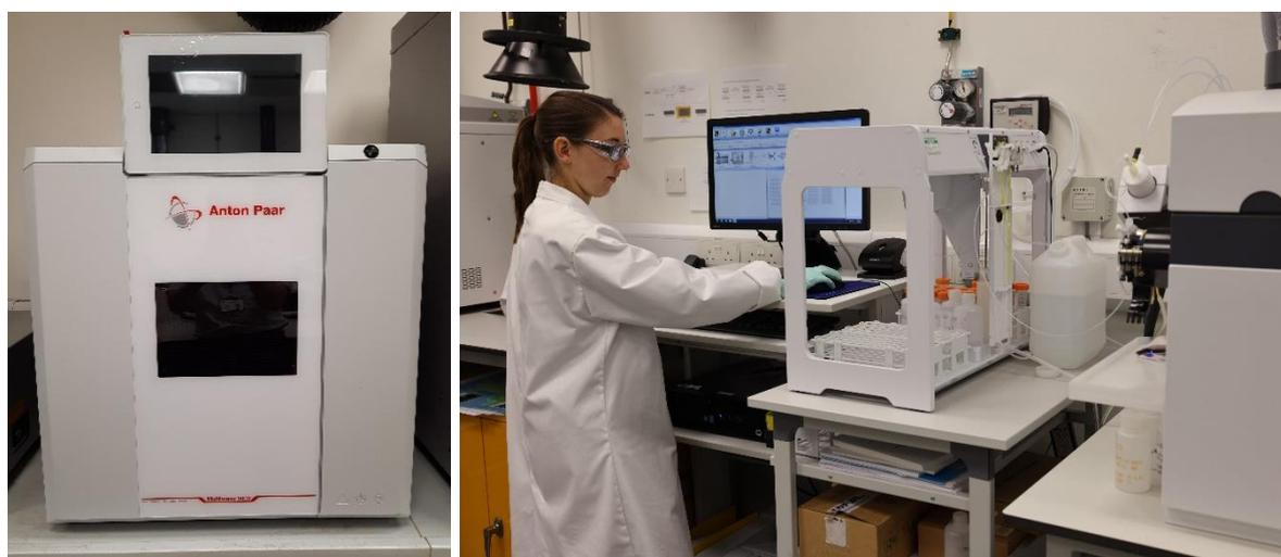
**Image 2 – (left) Anton Paar Multiwave 5000 microwave used for acid digestion of the sampled filters, (right) Agilent 8800 ICP-QQQ-MS in the UK ambient metals analysis facility at NPL.**
