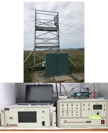
Figure 12 Photo of the Tekran set-up at Auchencorth Moss
