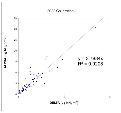
Figure 8: 2022 UKCEH ALPHA® uptake rate calibration
