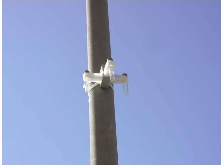
Figure 3: Example of how diffusion tubes can be fixed to a lamppost or similar.
