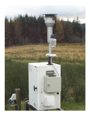
**Image 1.** The Partisol 2000 sampler at the Network monitoring site at Eskdalemuir. The grey box attached to the side of the sampler contains the mercury vapour sampling equipment (the particulate prefilter can just be seen protruding from the bottom right of the box.)
