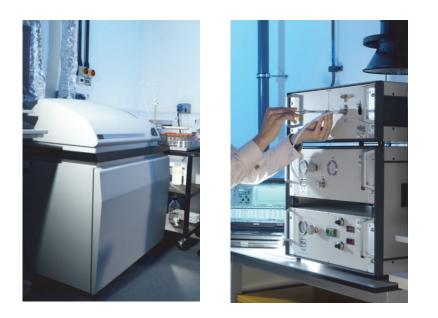
**Image 2:** (Far left) One of two dedicated ICP-MS instruments comprising the UK ambient metals analysis facility at NPL.
